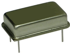
20.8 x 13.1 x 5.08mm Metal DIP Package
