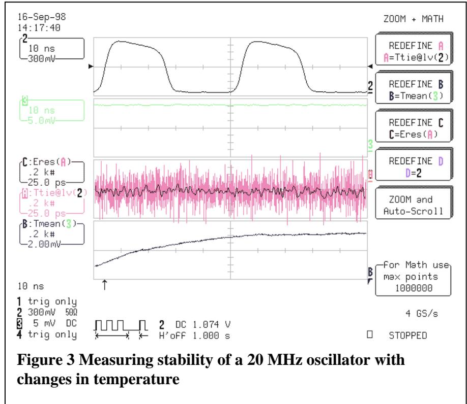
**Figure 3 Measuring stability of a 20 MHz oscillator with changes in temperature**
